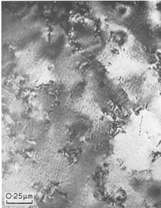
Figure 24 Contrast as observed in a stable \beta -phase Cu-48.5% Zn alloy containing only \omega -phase. This contrast is less pronounced than in a supersaturated \beta -phase also containing \alpha' component.
