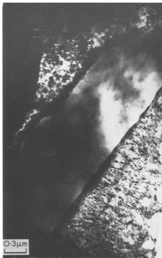
Figure 8 Retained \beta -phase in a Ag-39.1% Zn alloy pulse-heated to 348°C to form some Widmanstätten alpha-phase, then quenched. The \alpha -phase shows none of the mottled contrast evident in the surrounding phase.
