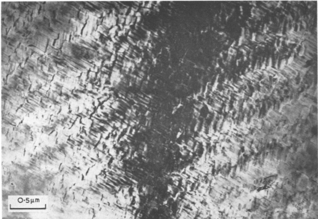
Figure 19 Typical \beta -phase contrast in a Ag-44.0% Cd foil oriented close to the \langle 111 \rangle_{\beta} axis.
