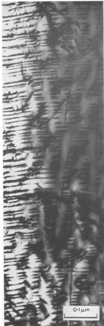
Figure 25 Precipitates in the massive \alpha_m -phase of a Ag-44.5% Cd alloy. The precipitates are in plate form parallel to \{111\}_{\alpha_m} planes. This HCP phase is most likely the equilibrium \xi -phase present in the Ag-Cd system.
