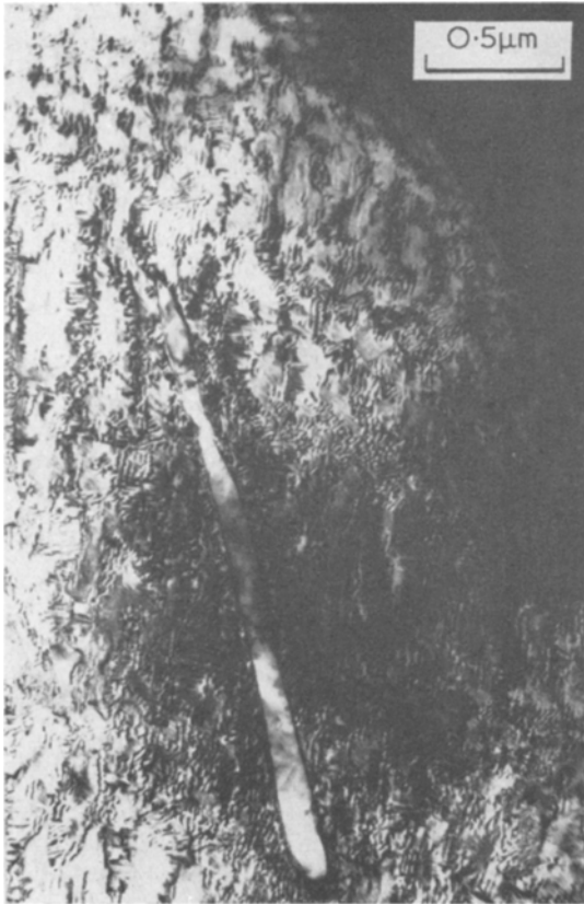
Figure 26 Moiré fringe patterns associated with large metastable precipitates in the supersaturated \beta -phase of a Ag-39.1% Zn alloy.
